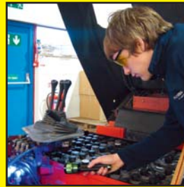
The system is scanned with either a Spectroline ultraviolet or UV/blue light inspection lamp.
